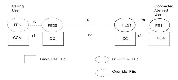
Figure 21 shows an example of the relationship between the model for SS-COLR and the model for the basic individual call. SS-COLR is available to the connected user (for connected line identification restriction).
